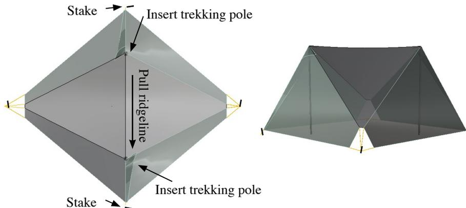
3. Now insert end pole tip into grommet or, if using taller trekking pole, into O-ring. While holding top of pole, remove end cording from initial stake and tension off to side as shown.
